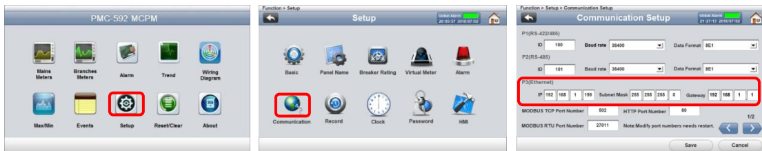
Figure 3-3 Configure PMC-592's IP Address
